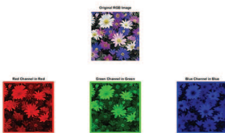
Figure 1: Original RGB image and its red, green, blue components.
