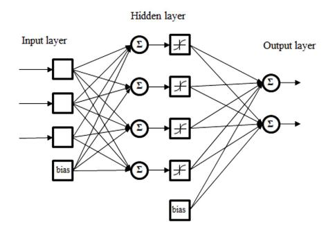
Figure 1: Feed-forward neural network model
